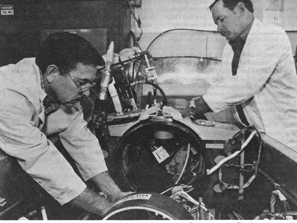
BOB PACHECO (left) and Larry Hill connect a weapon simulator to a B83 test system. Simulators are used to prepare for tests of actual systems, explains supervisor Len Parsons, because "tests on the real thing are — obviously — one-shot, and can't be repeated." Sometimes it takes days to prepare for an actual test that takes only seconds to run.
